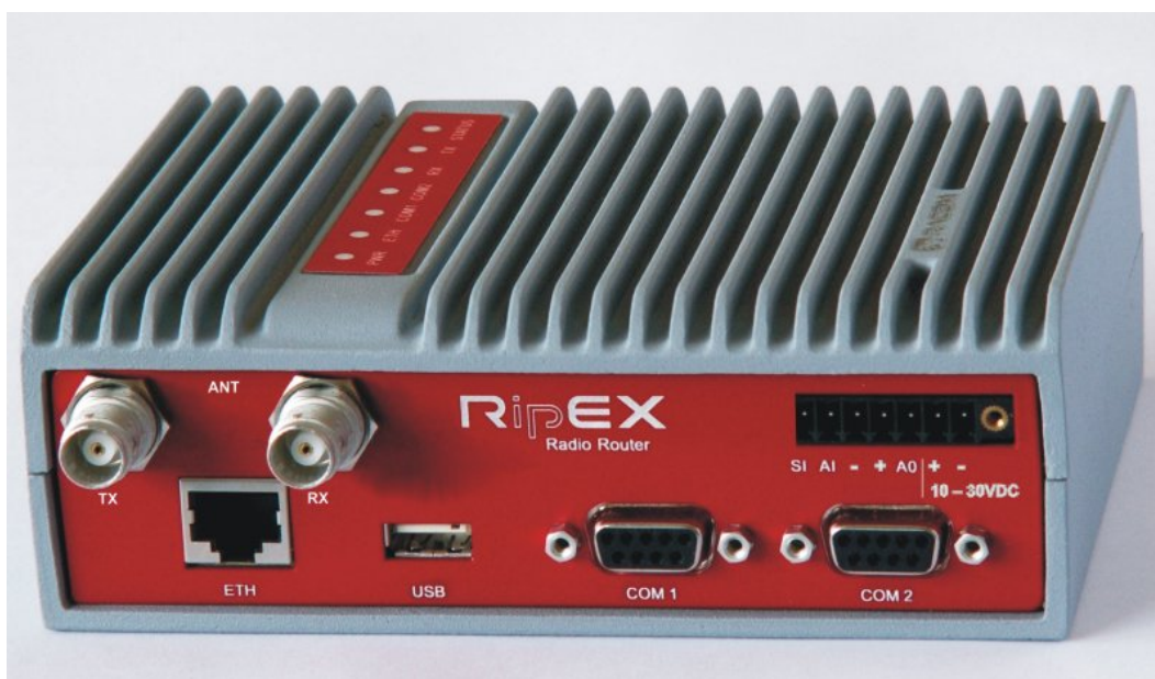
Fig. 4.7: Separated Rx and Tx antennas
