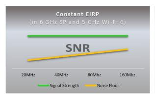
In 6 GHz SP class, the PSD measured in dBm/MHz matches the maximum EIRP on a 20 Mhz channel. Thus, as the channel width increases, the SNR decreases.
