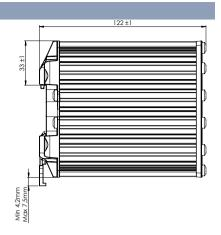
$134 \times 100 \times 122 \text{ mm} (5.25 \times 3.93 \times 4.80 \text{ in})$ Dimension
