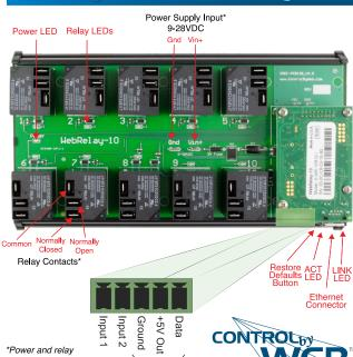
\*Power and relay connections require 1/4" push-on tab terminal connectors
