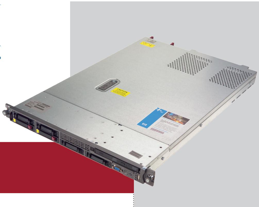
Viola M2M Gateway is connected to a fixed line internet connection by internet service provider. Viola M2M Gateway provides private and static IP addresses to Arctic devices. VPN tunnels are established and maintained between Viola M2M Gateway and Arctic devices.
