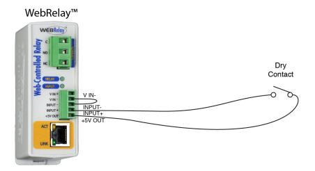
Many of the illustrations in this manual show the WebRelay contacts wired in series with a power source, which allows the power for the device to be switched on and off remotely. In many cases, however, it is useful to control other functions and not just power. One way to do this is to connect relay contacts in parallel with push-button switches within a device.
