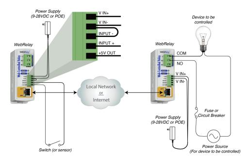
This configuration has may uses. It allows a switch to be placed a long distance from the device that it controls.
