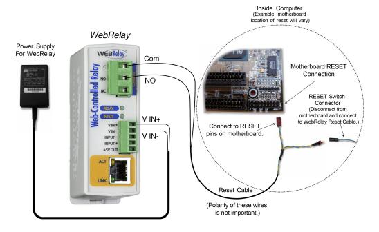
In this scenario, the computer is never powered down, only reset when necessary by temporarily closing the relay contacts. This approach is more gentle on the computer it controls than the approach of switching the power. The Common and Normally Open contacts of WebRelay are wired to the reset circuit of the computer. If the computer has an existing push-button switch for reset, the relay contacts may be wired in parallel with the push-button switch. This allows both local and remote reset.
