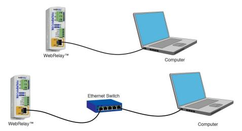
Connect the Ethernet port to a standard 10/100 Base-T Ethernet connection. The WebRelay typically connects to an Ethernet hub, switch, or router. The WebRelay does not support auto-negotiation on the Ethernet cable. For configuration, WebRelay may be connected directly to the Ethernet port on a computer using a "crossover" cable. Otherwise, for connection through a hub or router, a standard "straight-thru" cable should be used.
