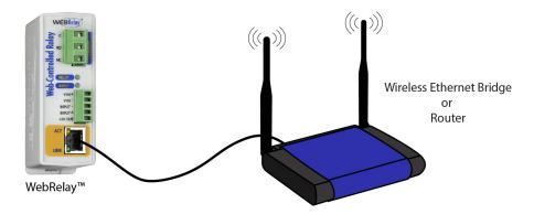
**Note:** The wireless Ethernet bridge or router must be properly configured for the wireless network. Refer to the installation instructions for the wireless device.
