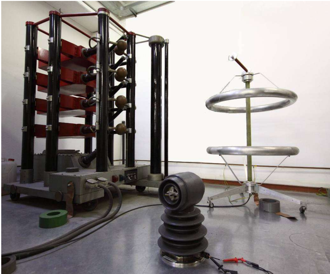
Impulse generator - up to 400 kV
