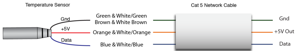
Figure 2.2i - Recommended connection using Cat 5 cable
