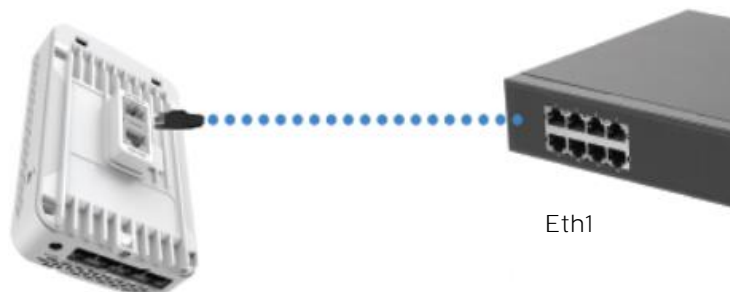
Figure 1 Installation of cnPilot to PoE capable switch
