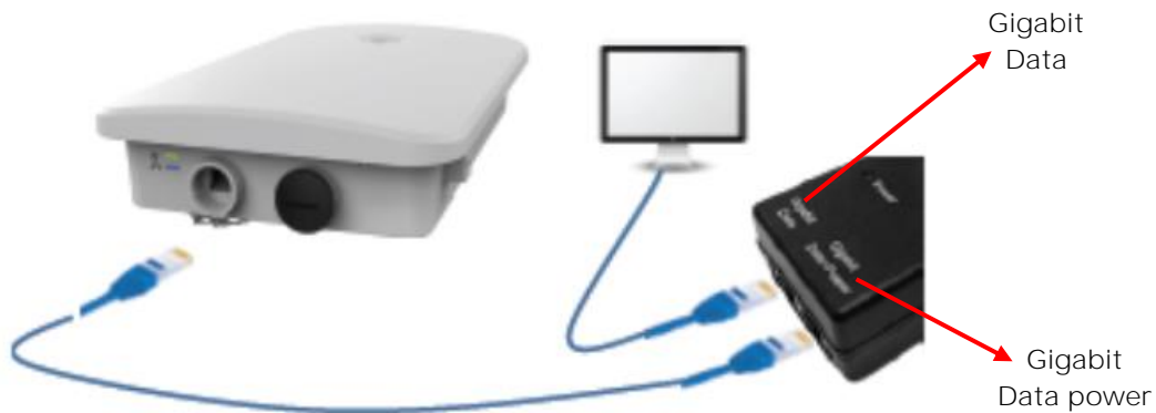
Figure 2 Installation of cnPilot to PoE adapter
