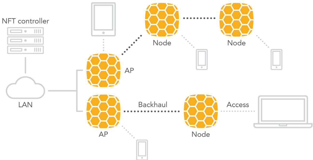
The main idea is to extend Wi-Fi coverage without using wires and to do that in an automated way without manual configuration.
