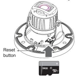
4. Open the SD card socket lid by sliding it backward and flip open the lid.
