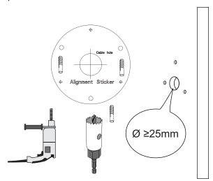
8. Route an Ethernet cable through the cabling hole.
