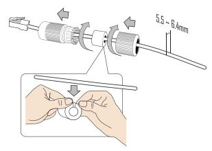
10. Install the seal ring and tighten the waterproof components.
