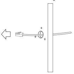
9. Pass an Ethernet cable through the waterproof cable gland components, and through the rubber seal as shown below. Connect the Ethernet cable to the camera's RJ45 connector.
