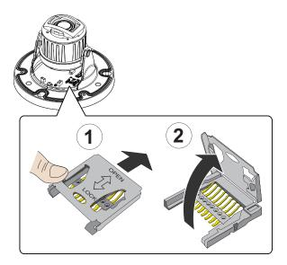
5. Insert a MicroSD card into the socket on the lid, with it's gold contacts facing down. Close the lid.
