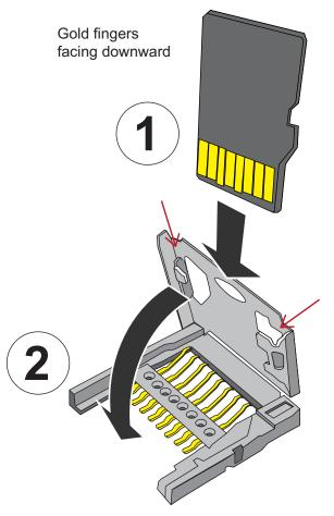
6. Slide the lid forward. A clicking sound should be heard to indicate that the lid and the card are secured in place.
