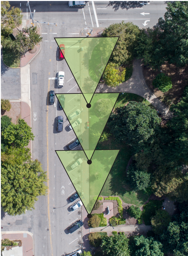
Figure 2: Example of overlapping fields of view to provide continuous analytics coverage of an extended area of interest.
