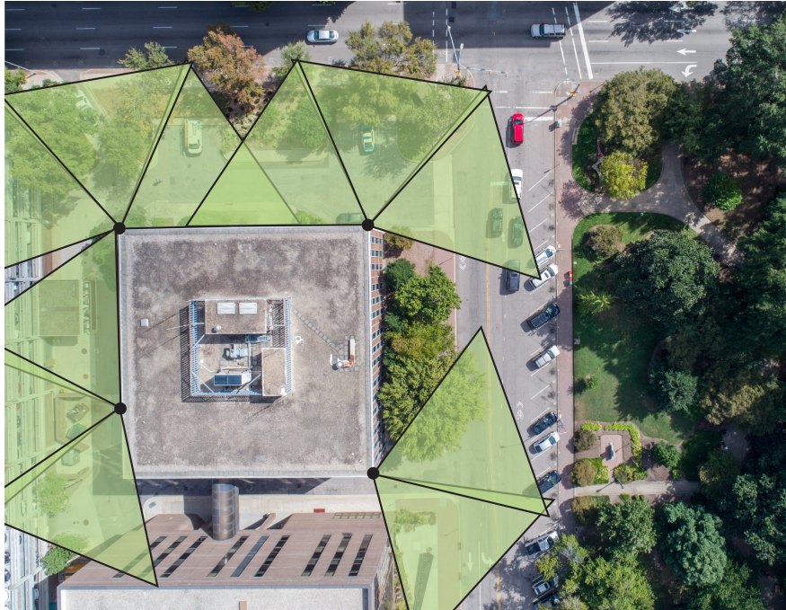
Figure 1: Example of overlapping fields of view for coverage of a building's perimeter.
