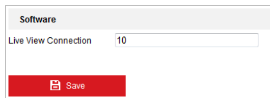
Figure 6-52 Live View Connection Settings
