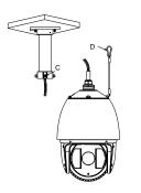
C: Safety rope hook  $\ \mbox{D}\colon$  Safety rope
