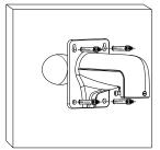
3 Tie the safety rope to hook and thread the cable
