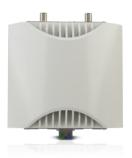
The Zinwave 3000 Distributed Antenna System (DAS) comprises centrally located Primary Hub units, distributed Secondary Hubs, and Remote Units deployed to provide wireless coverage throughout a building. The Primary and Secondary Hubs have the same form factor. The Remote Units are designed for un-obtrusive deployment on building walls or within ceiling voids.
