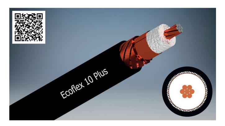
Ecoflex 10 Plus is an extremely flexible, low loss coaxial cable designed to use in the frequency range up to 8 GHz. Advanced manufacturing techniques combined with the use of a low loss PE-LLC dielectric with a foaming rate of more than 70% result in very low attenuation values, which set standards among flexible coaxial cables.
