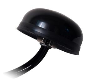
The Antenna-Roof-2L2W omnidirectional combo antenna for signal enhancement in mobile and WiFi networks. It can be used for weather stations, water supplies and much more. The antenna combines two LTE antennas and two WiFi antennas in a single housing and thus supports MIMO LTE/UMTS/GSM and MIMO WiFi 2.4/5 GHz. LTE and WiFi are linear polarized.
